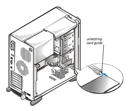
Figure 8-3. Unlatching the Card Guide
